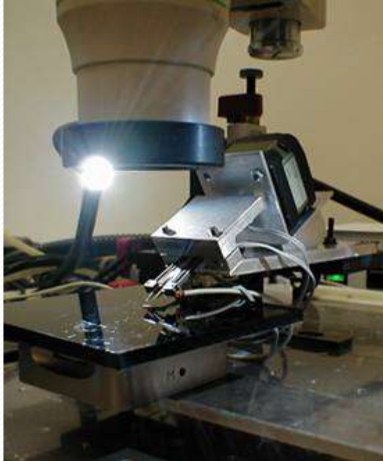
Basic configuration of two stages with piezo-motors 3 degrees of freedom each and a middle rotational stage.
